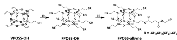
Scheme 2 Synthetic route toward alkyne functionalized fluorinated POSS (FPOSS-alkyne): (i) F8-SH, DMPA, \text{CHCl}_3 : TFT = 1 : 3, UV 365 nm irradiation, 30 minutes, r.t., 65%; (ii) 4-oxo-4-(prop-2-yn-1-yloxy) butanoic acid, DMAP, DIPC, \text{CH}_2\text{Cl}_2 : TFT = 1 : 3, r.t., 72%.
